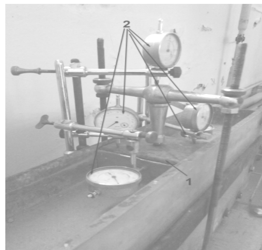
Fig. 8. Installing the lever system and indicators: 1 – a metal die; 2 – indicators of time type
