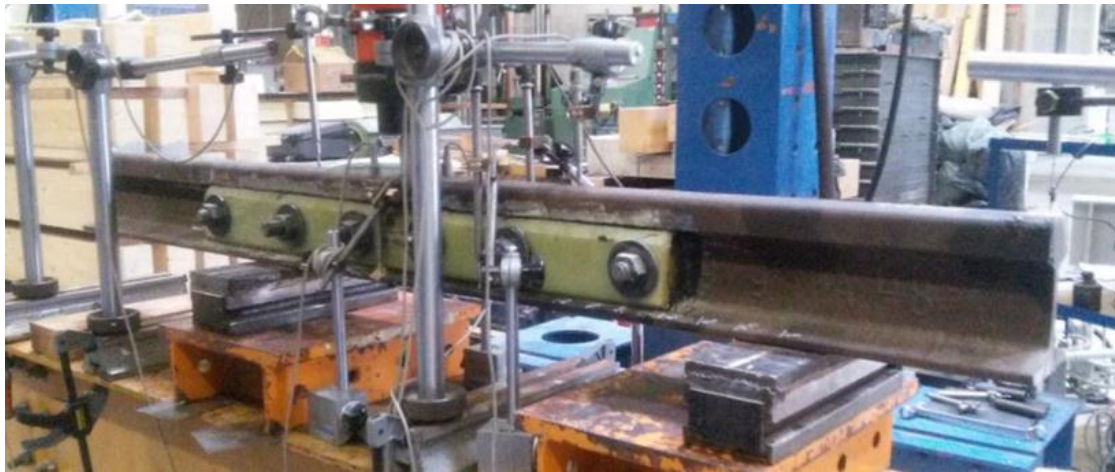
Fig. 2. The 3-point bending test arrangement of the laboratory measurement
