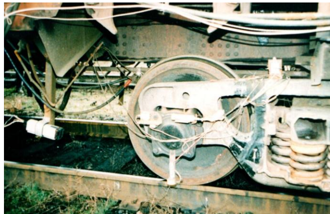
Fig. 9. Equipment of tested cars with measuring equipment: a – axlebox mount of the tested car with an acceleration and small displacement sensors; b – look of the tested standard car bogie;
