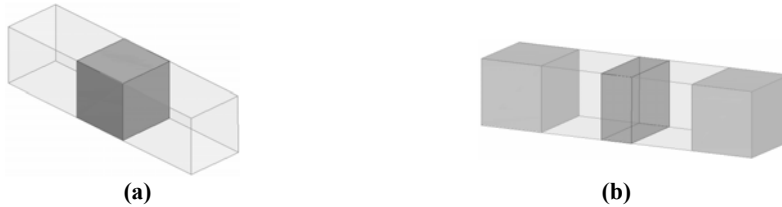
Fig.1. A waveguide-dielectric resonator model without its excitation device (a) and the variation of the cut-off waveguide excitation with dielectric filling inserts(b)
