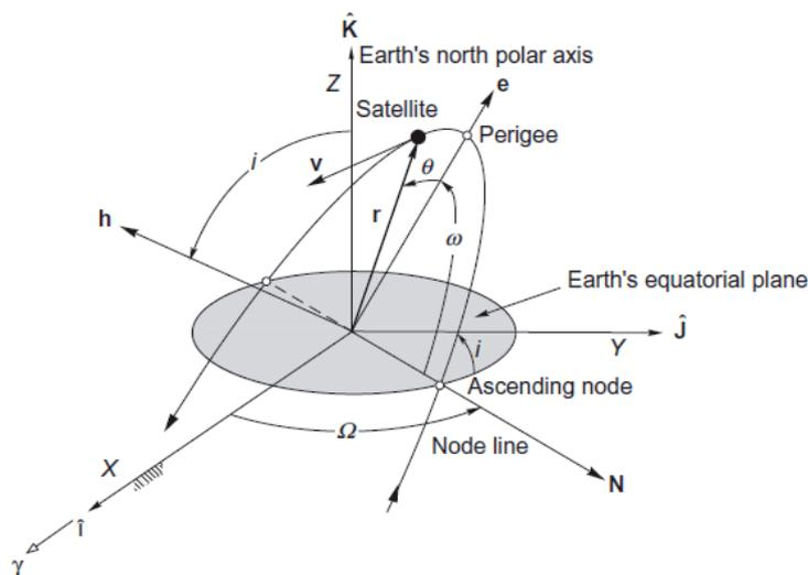
Fig. 1. Satellite orbital parameters (taken from [3])
