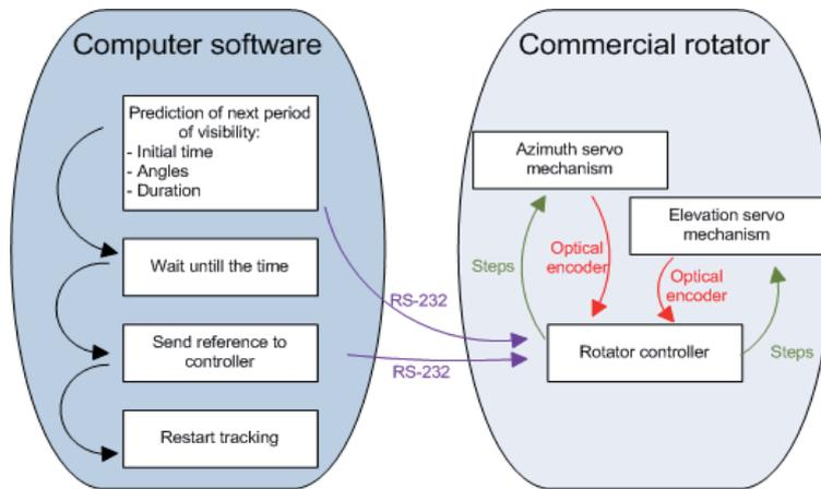
**Fig. 5. Controller schematics**
