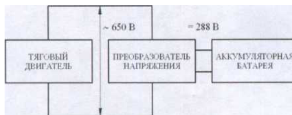
Fig. 1. The electric power car Lexus GS450h scheme
