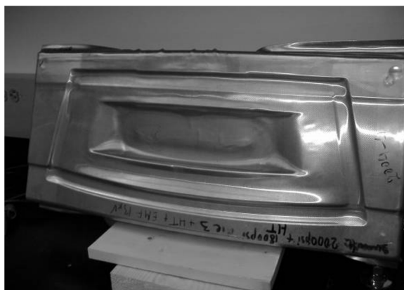
Fig. 1. – Car body part made by using magnetic-pulse stamping
