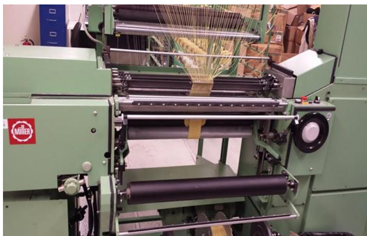
Fig. 3. Jacob Muller Warp Knitting Machine used for producing Auxetic Structures
