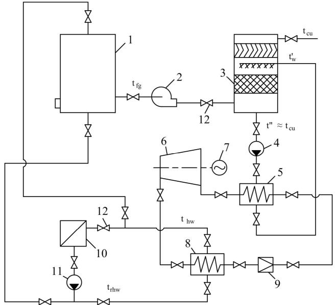
Fig. 1. Schematic diagram of utilization of flue gases heat from the boiler by means of recovery boiler and heat pumping installation: 1 – hot water boiler; 2 – smoke exhauster; 3 – contact recovery boiler; 4 – circulating pump; 5 – HPI evaporator; 6 – compressor; 7 –electric motor; 8 – HPI condenser; 9 – throttle valve; 10 – heat load; 11 – networking pump;12 – accessories
