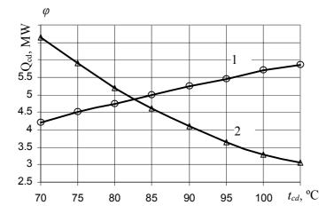
Fig. 2. Character of HPI condenser capacity and heating coefficient change
