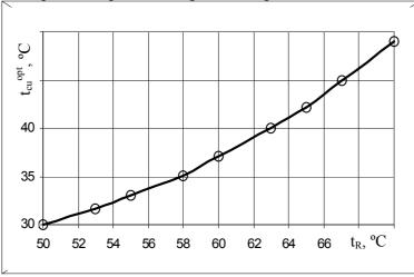
Fig. 5. Values of optimal cooling temperature of flue gases in contact recovery boiler
