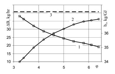
Fig. 4. Dependences of specific consumption of equivalent fuel for heat generation (curve 1) and value of equivalent fuel saving  $\Delta B$ ,  $\kappa g/h$  (curve 2)
