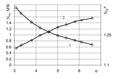
Fig. 3. Current values of HPI compressor capacity (curve 1) and relative power of the heating pump (curve 2)
