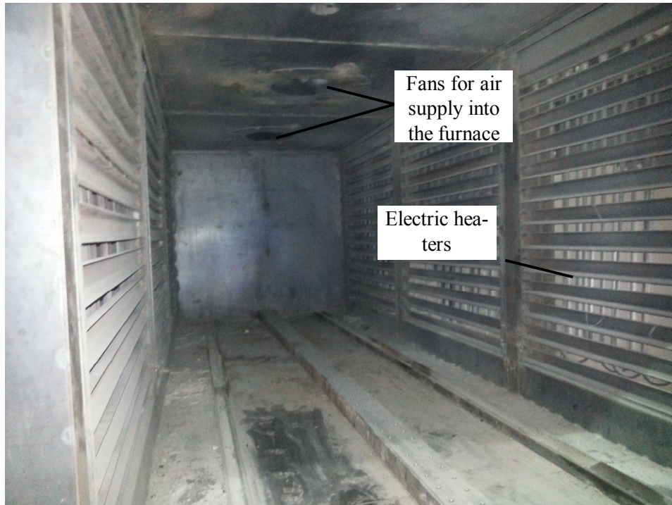
Fig. 1. Internal construction of the furnace
