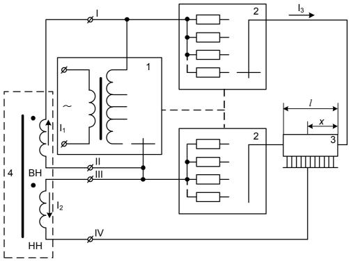
Fig. 1. Diagram of the device for determination of transformation ratio of the transformers
