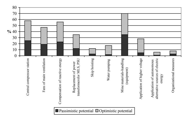
Fig. 2. Comparison of optimistic and pessimistic potentials of energy efficiency increase of the elements of the systems of energy supply and electric equipment of iron-ore mines
