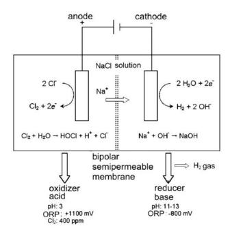
**Fig. 1**. The diaphragm electrolysis method for the preparation of acid (anolyte) and alkali (catholyte) solutions via the electrochemical activation of sodium chloride
