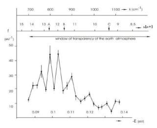
Fig. 4. NES-spectrum of deionized water (chemical purity – 99,99 %; pH – 6,5–7,5; total mineralization – 200 mg/l; electric conductivity – 10 μS/cm). The horizontal axis shows the energy of the H...O hydrogen bonds in the associates - E (eV). The vertical axis - energy distribution function – f (eV<sup>-1</sup>). k – the vibration frequency of the H–O–H atoms (cm<sup>-1</sup>);  $\lambda$  – wavelength ( $\lambda$ m).
