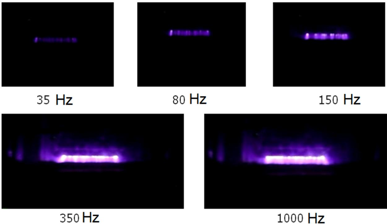
**Figure 4 - Photos of the nanosecond discharge with the electrode based on distilled water (view from the side of electrode) at the various voltage repetition frequencies at the distance between edges of blades and water surface of 7,5 mm and the thickness of water over the solid metal electrode of 4 mm**
