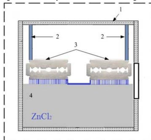
**Fig.2** - The structure of discharge cell with rotary electrodes: 1 - cuvette made of organic glass, 2 - regulating electrode screws, 3 - blades, 4 - distilled water or control salt solution of zinc chloride ( $ZnCl_2$ ) in water.
