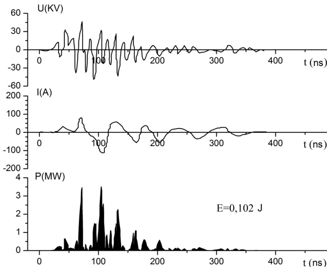
Figure 6 - Temporal dependences of the voltage, current and power of the nanosecond discharge (discharge over the surface of distilled water) at the distance between electrodes of 25 mm.
