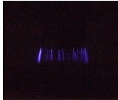
**Figure 3 - Photos of the nanosecond discharge with the electrode based on distilled water (view from the end of electrode) at the voltage repetition frequency 40 Hz at the distance between edges of blades and water surface of 7,5 mm and the thickness of water over the solid metal electrode of 4 mm**
