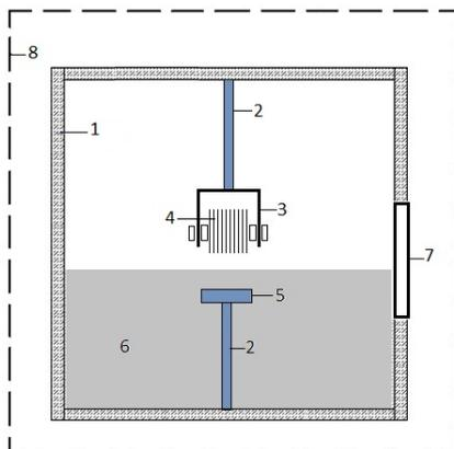
**Fig.1** - The structure of discharge cell: 1 – cuvette, 2 - screws for installation of interelectrode distance, 3 - mounting of electrode, 4 - blade system, 5 - metal electrode dipped in water, 6 - distilled water, 7 - quartz window, 8 - metal screen
