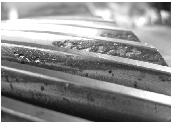
Fig. 5. Typical defects of gearwheel caused by improper centering
