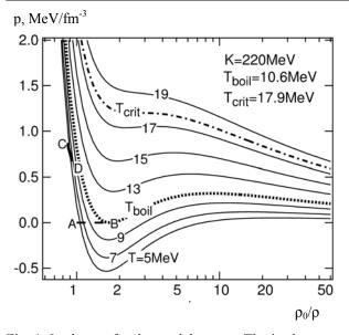
Fig. 1. Isotherms for the model matter. The isotherm corresponding to zero-pressure boiling-point temperature is shown in dotted line and the critical isotherm is shown in dash-dotted line. The adiabatic thermal expansion trajectory for the system at zero-pressure is shown in dashes as line AB, with B being the boiling point. The bulk interior expansion trajectory for finite system is shown in bold solid line CD.
