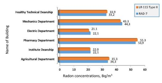
Fig. 2. Comparison of RAD-7 and LR-115 Type II results. (See color Figure on the journal website.)
