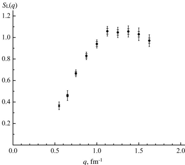
Fig. 2. Experimental Coulomb sum values of  ${}^7\text{Li}$ . The error bars at the points represent the sum of systematic and statistical uncertainties. The systematic uncertainties are shown by a wide cap on the line of the summary error bar.
