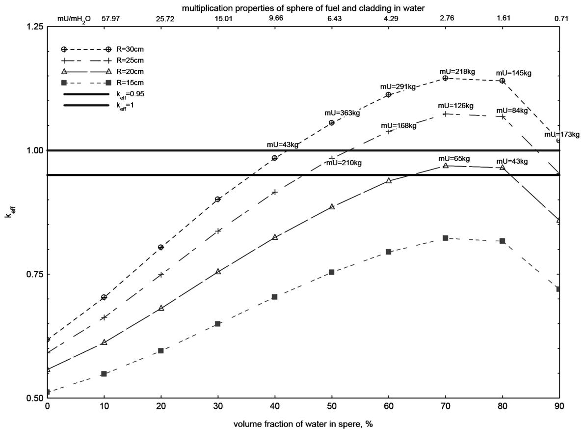
Figure 11 – criticality of fuel and claddings in water
