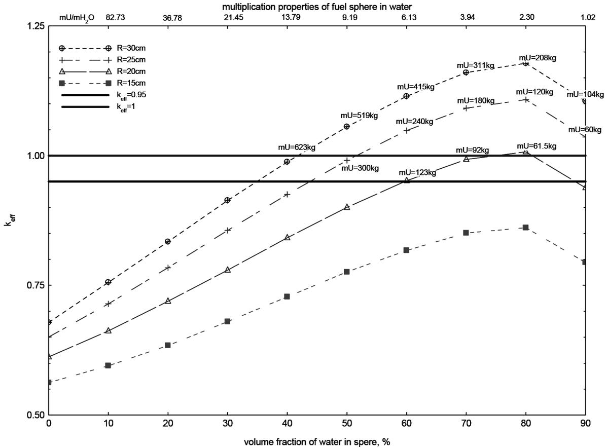
Figure 10 – criticality of fuel in water
