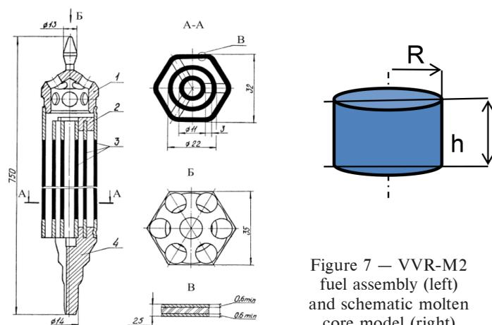
Figure 7 — VVR-M2 fuel assembly (left) and schematic molten core model (right)
