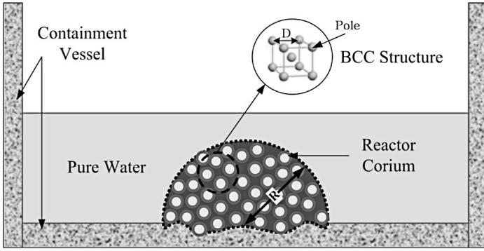
Figure 3 — conceptual model for criticality calculation from [8]
