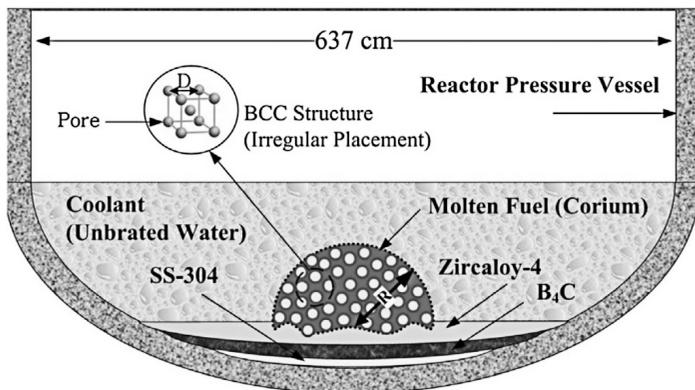
Figure 4 — conceptual model for criticality calculation from [9]
