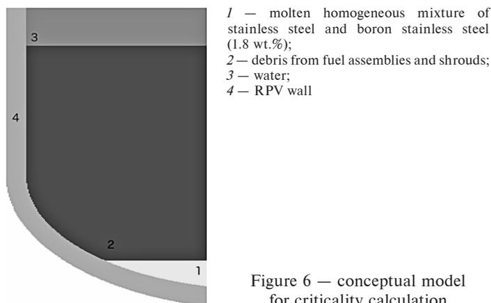
Figure 6 — conceptual model for criticality calculation
