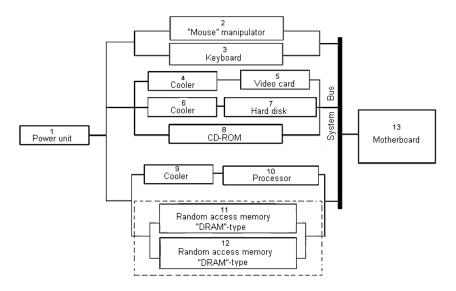
Figure 2 – Simplified block diagram of a typical PC
