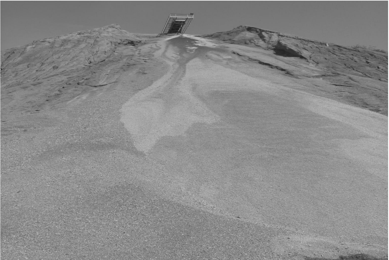
Fig. 1. General view of display of segregation on-the-spot of dump.
